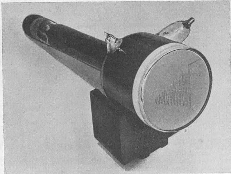
Fig. 6. British dark trace tube with trace on screen
