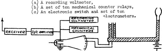
The mechanical counters (b) were of P.O. type and each was arranged by means of magnetron relays to operate whenever the f.s. exceeded the specified value corresponding to that particular counter. Specified values corresponded to .5, 1.0 .. 5.0 v/m. The numbers were counted every 15 minutes.
