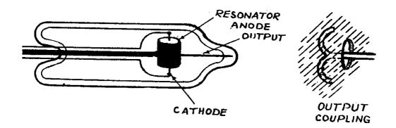
The exact mode of operation of the magnetron was not clearly understood but it was stated that for optimum efficiency the length of the cavity should be 0.85 times the diameter (internal dimensions).
