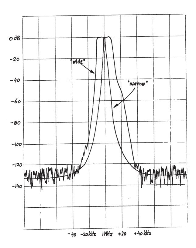
Actually plotted IF over-all response curve of the receiver owned by the Author. The slight assymmetry is probably caused by a detuned roofing filter (the circuit has not been trimmed since almost half a century ago...).
