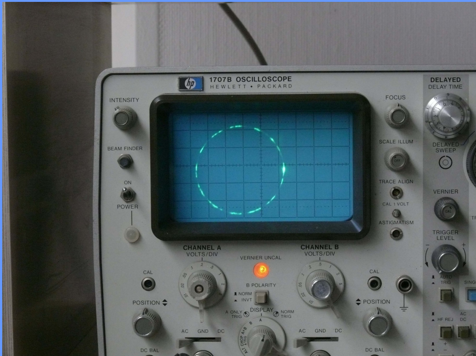
A nice example of a combined screen display of a coherent signal spot and a non coherent EGON signal (dashes 2 Hz PRF difference)
