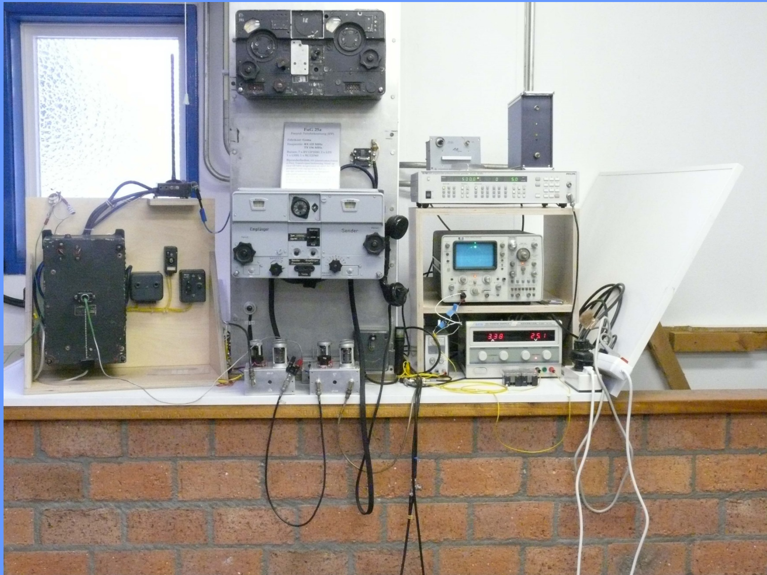
Hypothetical aircraft Nachtfee setup, but fully HF operational
